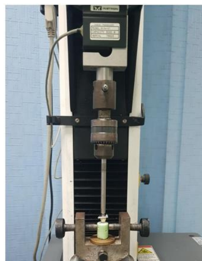
Figure (3): Fracture resistance test of a sample using Instron testing machine.
