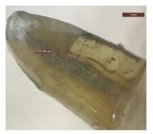
**Fig. 3:** Stereomicroscopic images of samples with the depth of methylene blue dye penetration
