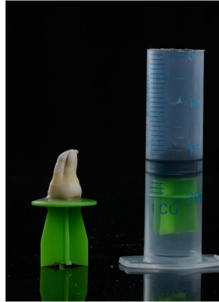
Figure 1: Extracted tooth mounted in a custom jig for standardized positioning before embedding in epoxy resin mold.
