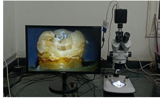
Figure 5: Fractured specimen after static load testing, showing a Class IV longitudinal fracture involving both the restoration and tooth under a stereomicroscope.
