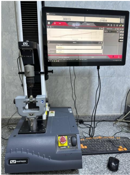
Figure 4: Specimen fixed in Universal testing machine for fracture load testing.
