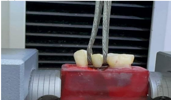
(Figure4): (A,B) Debonding Test using Universal Testing machine
